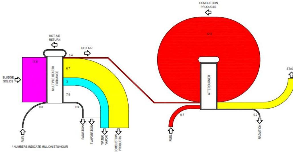
In any biosolids incineration system the bulk of the input energy is derived from the combustion of VS and fixed carbon in the biosolids feedstock. If the heat energy produced by the thermal oxidation of carbon and VS is not sufficient to evaporate the water in the feedstock, then auxiliary fuel is added to the MHF or FBC incinerator. Autogenous or self-sustaining combustion has been achieved in both the MHF and FBC at about 28% to 30% Total Solids (TS) and about 75% to 80% VS.
