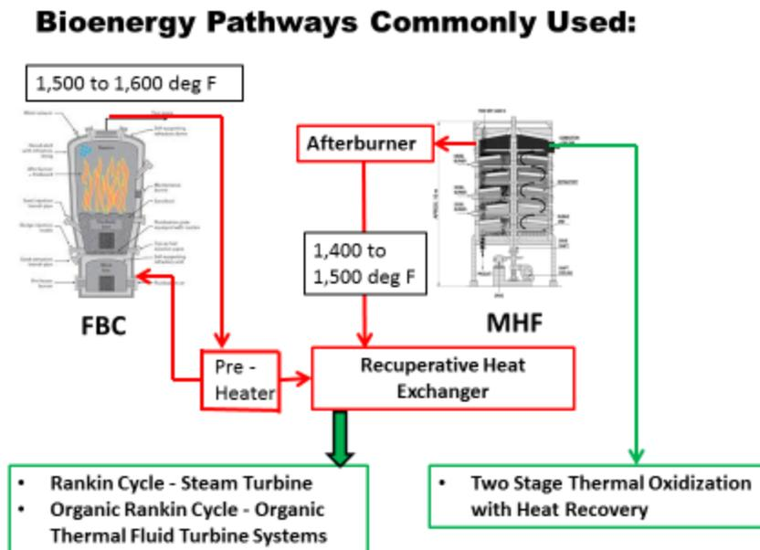
**Figure 2 Rankine Cycle Energy Recovery**
